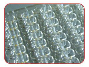
Drop volumes of up to 10  $\mu$ l are possible. The 9 mm standard distance between wells is preserved, enabling the use of multi-channel manual pipettes and robotic liquid handlers, making MRC Maxi one of the most automation-friendly optimisation plates on the market.
