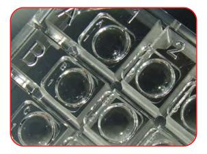
The SWISSCI MRC Under Oil 96 Well Crystallisation plate uses oil as a seal and active diffusion mechanism for the purpose of running macromolecular crystallisation under oil. Following the initial experiment, the solution under the oil is sequentially allowed to evaporate as a second stage enabling further crystal growth as a consequence of concentration. This is different from other experiments in that the conditions are then extreme in nature and permit new conditions to arise.
